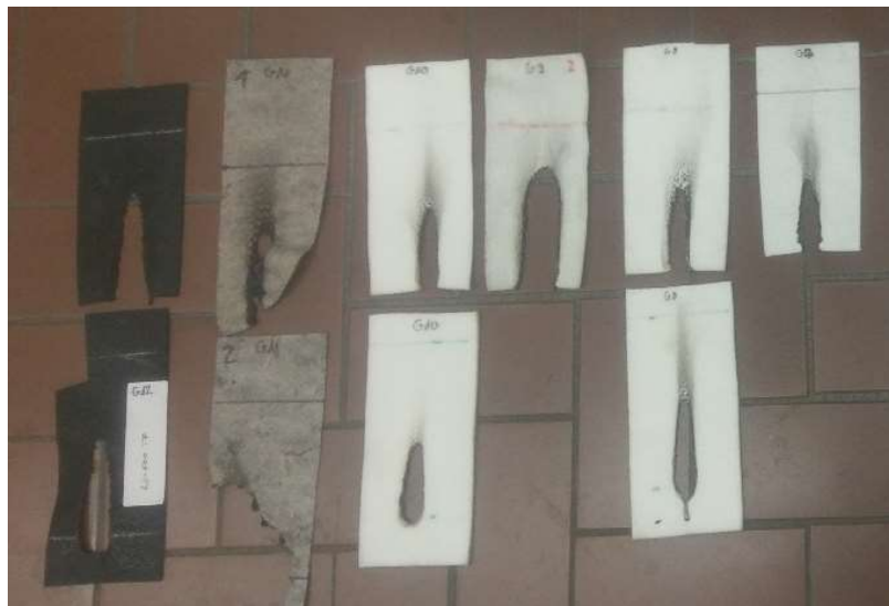
4. Figure: Damage to samples G7-G12 after wind and surface ignition
