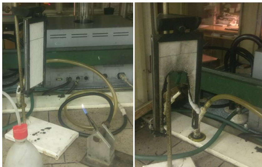
1. Figure: Vertical flame spread speed testing equipment and their combustion in case of wind ignition
