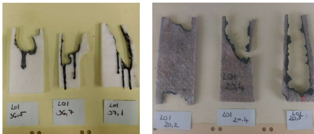
6. Figure: Damage of samples G8 and G11 burned in different oxygen contents
